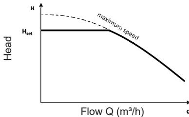
Figure 9.5: The curve of the Variable Pressure Mode
