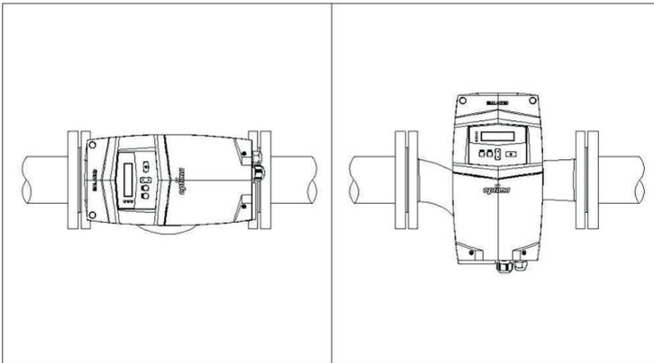
Figure 5.3: Control Box Position Adjustment
