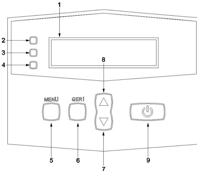
Figure 7.1: Control Display Layout
