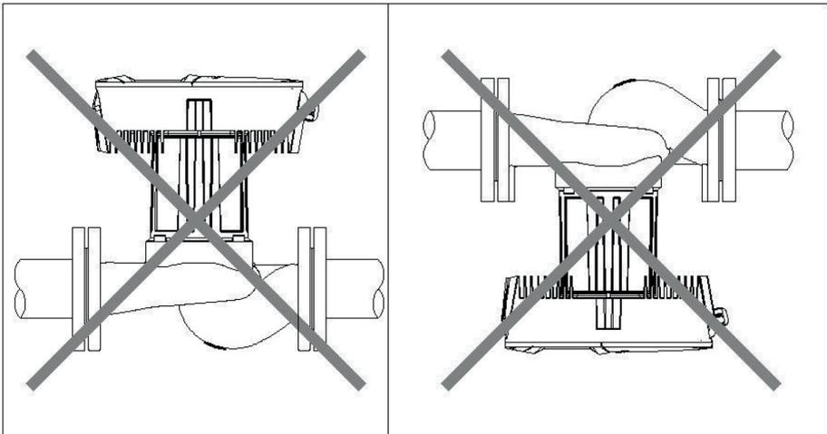
Figure 6.2: Incorrect Pump Positions
