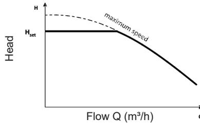
Figure 9.3: The curve of the Constant Pressure Mode
