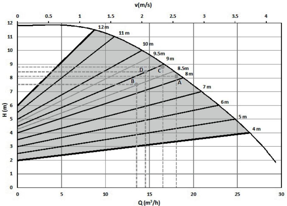
Figure 9.6: Example of the Variable Pressure Mode
