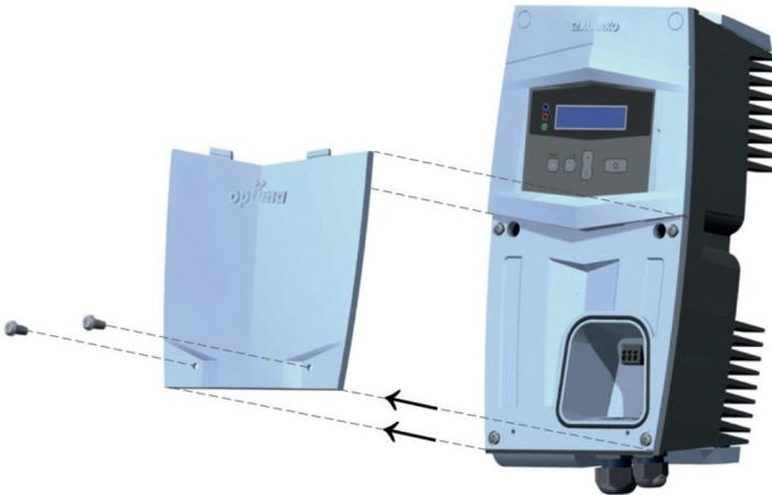
Figure 6.8: Removal of the Bottom Cover
