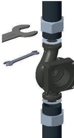
Figure 6.4: Threaded Pipe Connection
