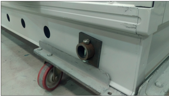
Fig. 7. Fastening of Lifting Bars - 3
