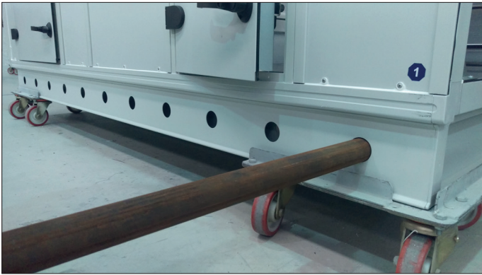
Fig. 6. Fastening of Lifting Bars - 2
