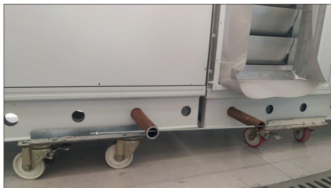
Fig. 12. Connecting the sections using threaded bars
