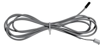
Type NTC sensor, to be placed on the water supply pipe upstream 3 way valves (not to be used with 2 way valves).
