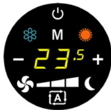
The CB-Touch control allows to control and adjust the room temperature in a simple and intuitive way by means of a probe positioned in the lower part of the unit.
