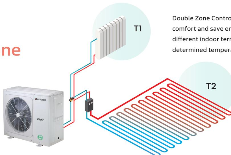
Double Zone Control can be used to increase comfort and save energy by ensuring that different indoor terminal units operate at determined temperatures.
