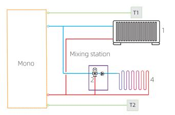
Notes: 1. Radiator (field supplied) 2. 3-way valve (field supplied) 3. Water pump (field supplied) 4. Floor heating loop (field supplied) Abbreviation: T: Room thermostat (field supplied)
